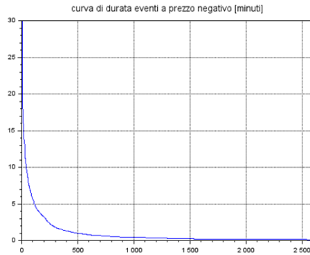
Figure 23 Duration curve of negative price events with a duration of more than 4 seconds
